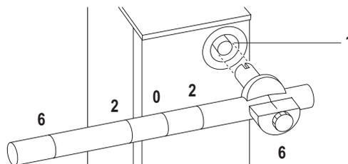
Fig. 12: Check e.g. at measuring drum setting 6
